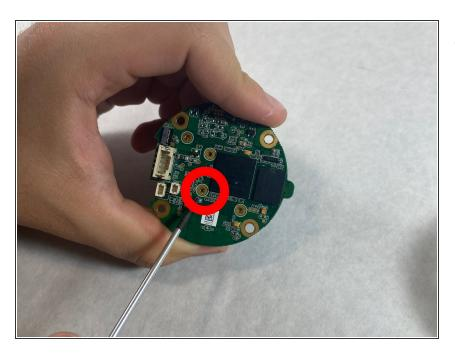
• Remove the four mounting screws from the motherboard.
