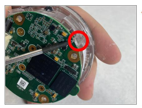
Pry the plastic cover away from the motherboard at the plastic clips using a spudger.
