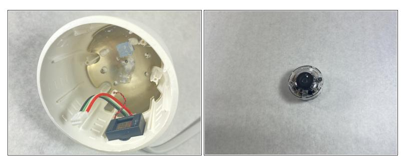
• Remove the plastic camera cover from the device.
