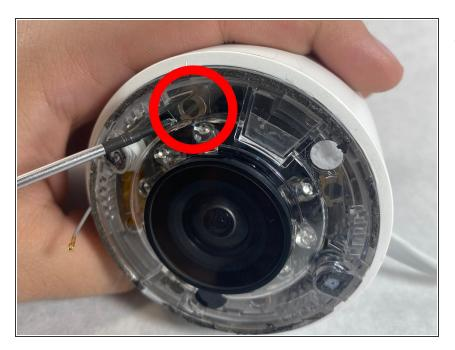
• Remove the four small screws from the plastic camera cover.
