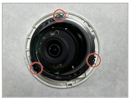
Remove three screws that connect the camera base to the motherboard using a Phillips #1 screwdriver.
