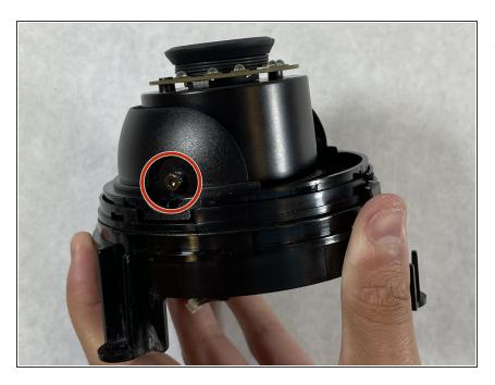
Unscrew the camera from the camera base with a hex screwdriver on both sides.
