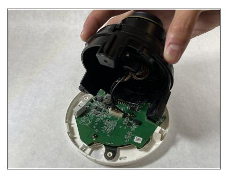
• Lift off the camera base from the motherboard.
