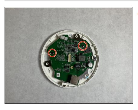
Once the camera module is removed, unscrew the two remaining screws which attach the motherboard to the backplate.
