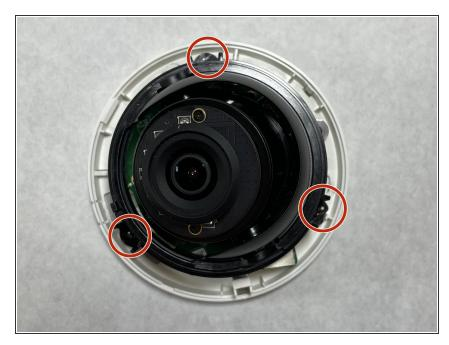
Remove three screws that connect the camera base to the motherboard using a Phillips #1 screwdriver.
