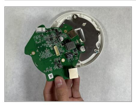
Once the screws are gone, lift the faulty motherboard and replace with a new one.
