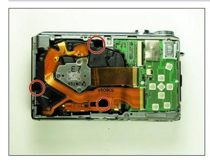
Remove the three 3 mm black screws that surround the lens using a Phillips #00 screwdriver.
