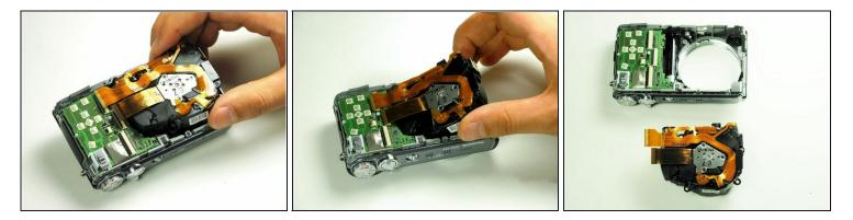
• Use your fingers or a spudger to gently remove the lens mechanism from the rest of the camera.
