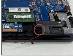
Using the Phillips #0 screwdriver, remove the two screws (one on each speaker) securing the speakers to the motherboard.
