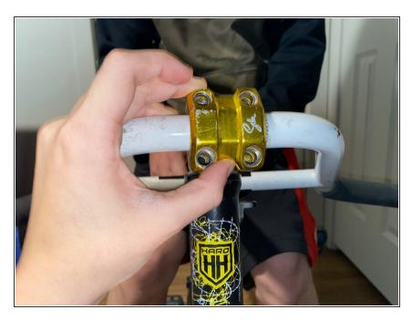
Place the faceplate of the stem back on and align the screw holes.
