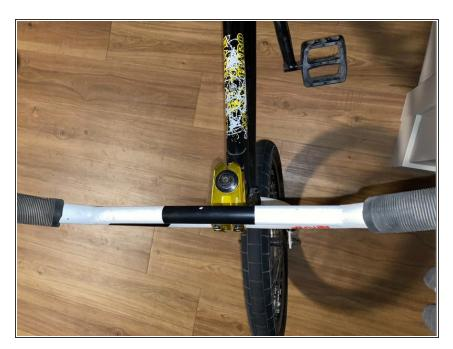
Locate the stem of the bike connecting the handlebars to the steerer tube of the fork.
