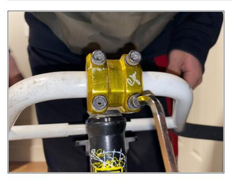
Insert the four screws back into the stem and tighten them half way with the 6mm Allen wrench.
