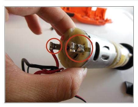
Wait for the wires and connectors to cool. Pull the wires from the motor and the motor should now be fully disconnected from the drill.
