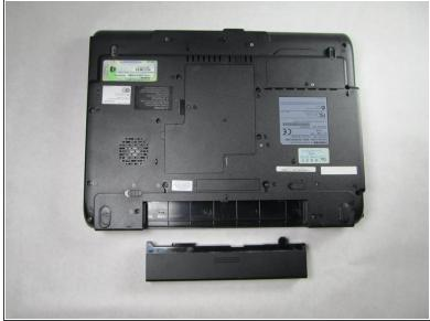
Hold the release switch and pull out the battery towards you.
