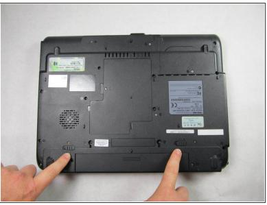
Turn the laptop over and locate the lock and battery release switches. Unlock the battery by changing the switch on the right from locked to unlocked by sliding the switch outward.
