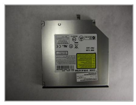
i This disk drive model appears to not have any connecting wires, however your disk drive might need additional steps to connect it to the motherboard.
