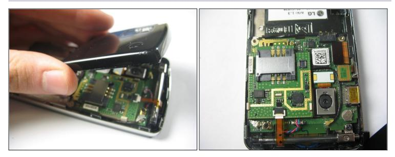
• Remove the plastic case to reveal the motherboard.
