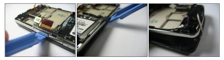
• Insert a plastic opening tool below the volume rocker and gently pry the silver casing up. As with the plastic casing over the motherboard, you should be able to slide the plastic opening tool along the edge to remove it.
