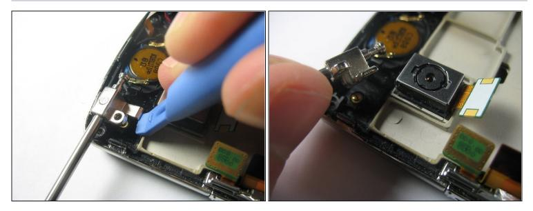
• Use a plastic opening tool to carefully pry up the metal antenna guide.
