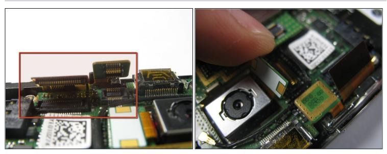
• Remove the remaining three ribbon cables by gently lifting them by the ends, opposite of the cables, with a plastic opening tool or spudger until they pop out.
