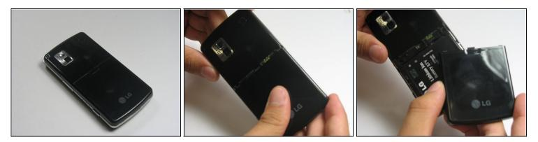
• Remove the back cover by firmly pressing against the indent on the back panel. Slide the cover downward and off the phone.
