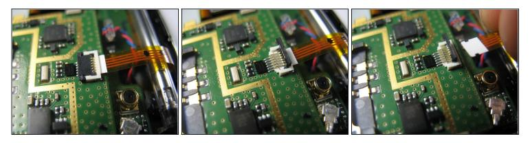
• Gently lift the ZIF connector (black tab) holding the ribbon cable in place. When it is in the upright position, remove the cable from the back side.
