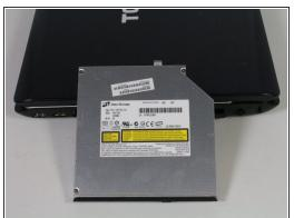
Continue to pull the disk drive toward you until it is completely removed from the laptop's housing.
