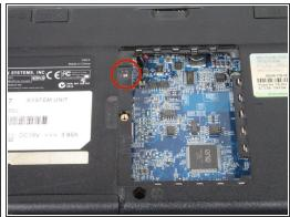
Remove one 1.5mm Phillips #1 screw located near the top left edge of the opening.
