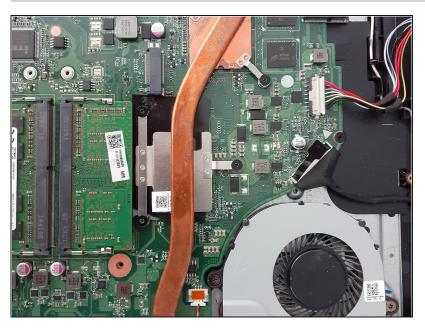
Put the heatsink back on and screw it in place.
