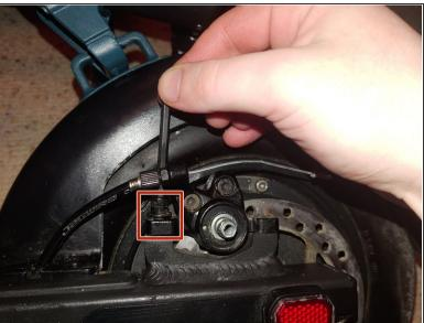
Use the 4 mm Hex key to remove two 22 mm screws that hold the caliper to the scooter body.
