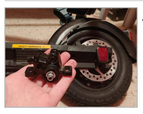
Remove the brake caliper.
