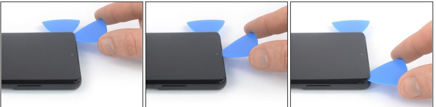
**⚠** When you slice near the front facing camera, insert only the tip of the opening pick (~2-3 mm) to avoid damaging or smearing the camera.
