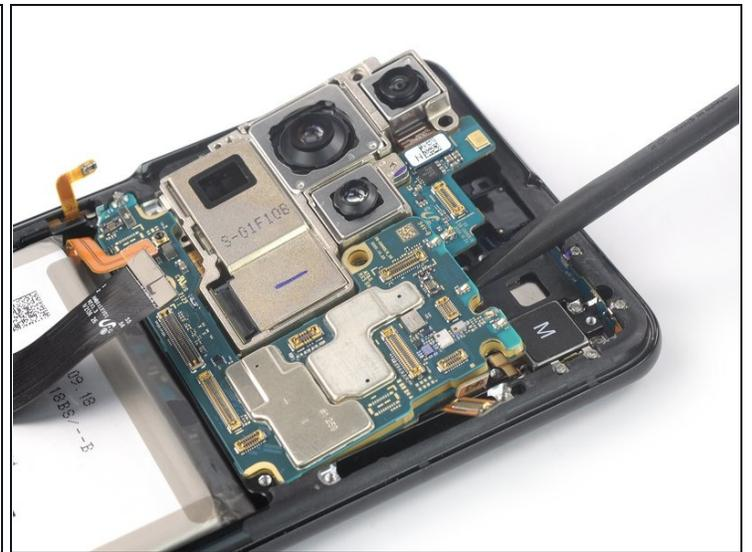
**⚠ Avoid damaging the flex cables surrounding the motherboard during the following procedure.**
