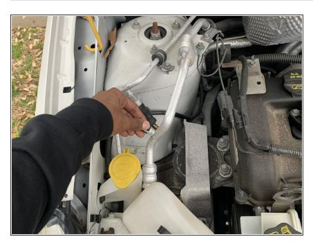
Remove the cap by turning it counter-clockwise.
