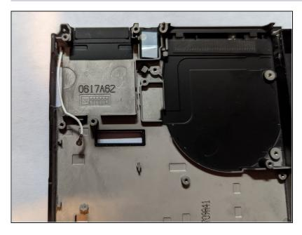
Verify the coax wire is free of any obstructions or routing inside the device.
