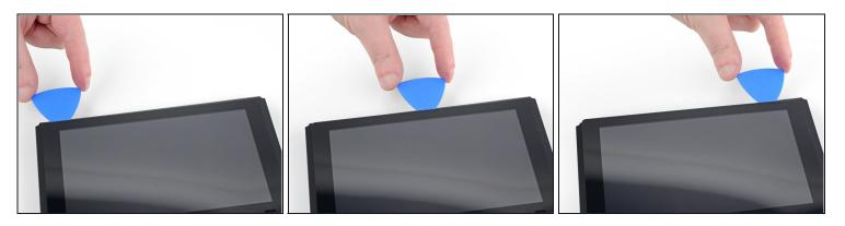
• Continue sliding the opening pick along the top edge of the screen to slice the adhesive.
