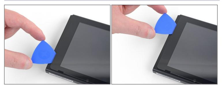
• Continue sliding the opening pick along the left edge of the screen to slice to adhesive.
