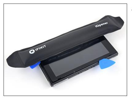
Heat the top edge of the screen for around two minutes to help soften the adhesive.
