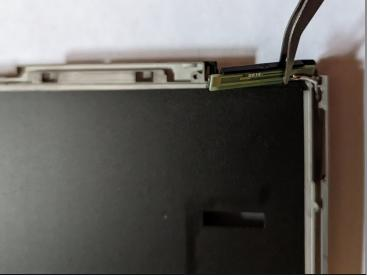
• The antenna is held in with light adhesive, so simply grasp it and pull up to release it.
