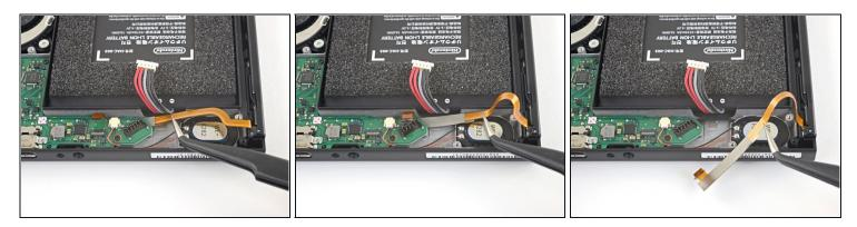
• Use your fingers or a pair of tweezers to lift the battery connector up and out of the way of the Joy Con rail's data cable.
