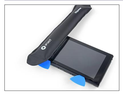
Heat the left edge of the screen for around two minutes to help soften the adhesive.
