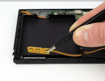
• Remove the power/volume board with a pair of blunt nose tweezers.
