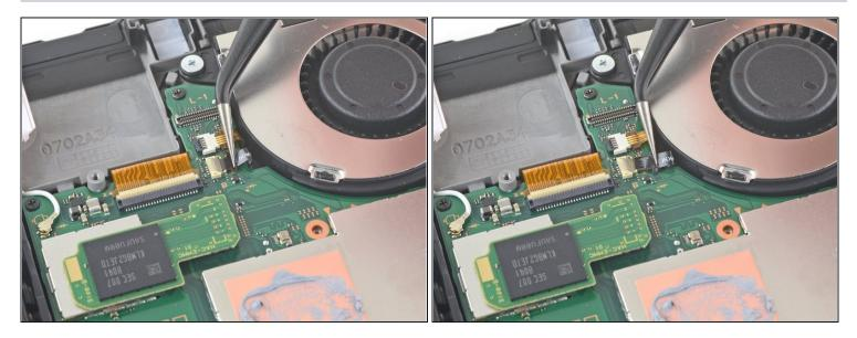
• Use a pair of tweezers to pull the fan cable straight out of its connector on the motherboard.
