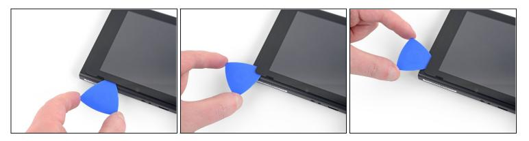
• Continue sliding the opening pick around the bottom-left corner to slice the adhesive.
