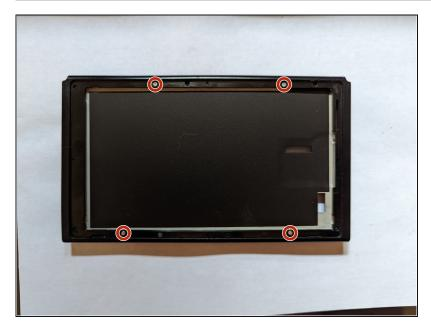
Remove the four screws securing the front frame to the midframe.
