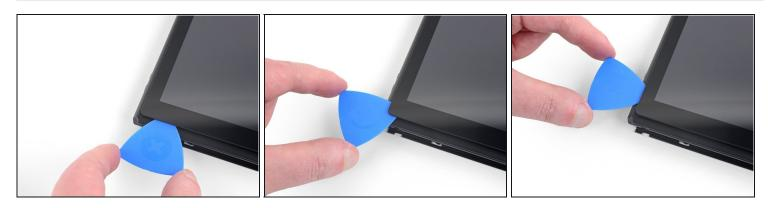
• Continue sliding the opening pick around the top-left corner of the screen to slice the adhesive.
