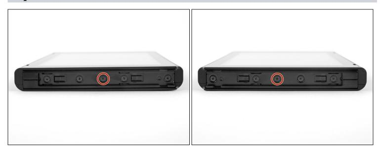
• Use a JIS 000 screwdriver or an official iFixit PH 000 driver to remove the two 3.8 mm center screws on the sides of the device (one on each side).
