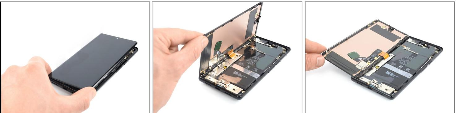
**⚠ Avoid straining the display cable during the following procedure.**
