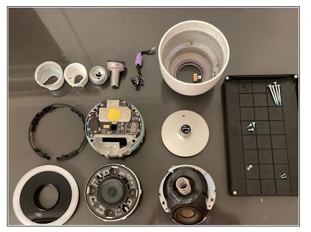
You are now done disassembling the unit to the module level! Check out the other guides (coming soon) to see how to break down the modules further.
