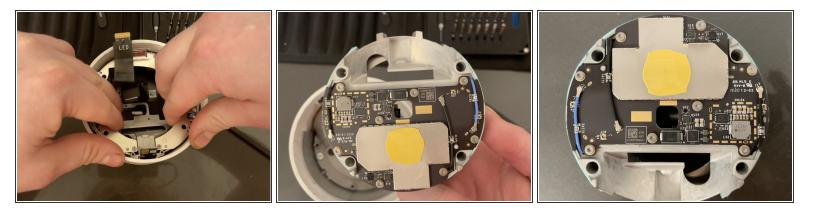
• Using both hands, gently pull upwards making sure the power cable, speaker cable, and power pad route down through/around the motherboard module as you pull it upward.
