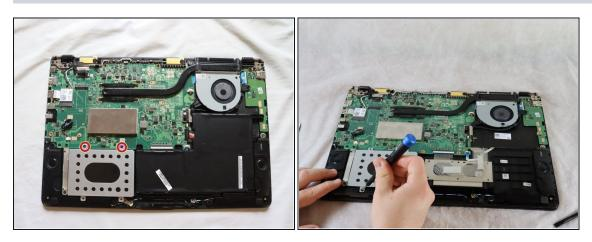
• Remove the two 4 mm Phillips #1 screws which are holding the hard drive cover in place.
