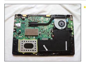
The hard drive is located to the left of the battery and below the motherboard.
