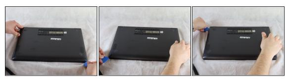
• Use an opening pick to separate the back cover from the device.
