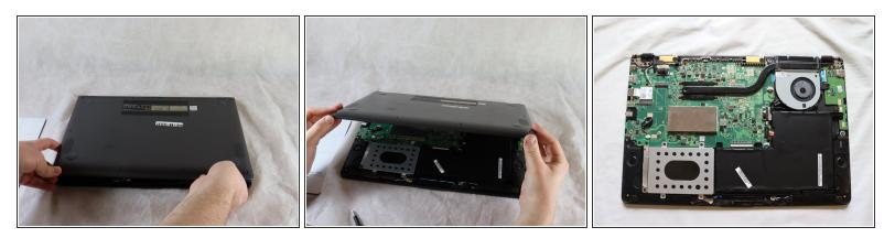
• Once the cover has been separated from the device, carefully lift the back cover off the device (begin by lifting from the front of the cover first).
