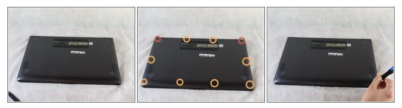
A Begin by powering off the device and flipping the device over.
