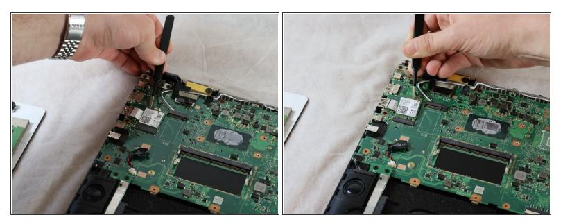
Use the pointed tweezers to pull the network card out and away from the socket.
