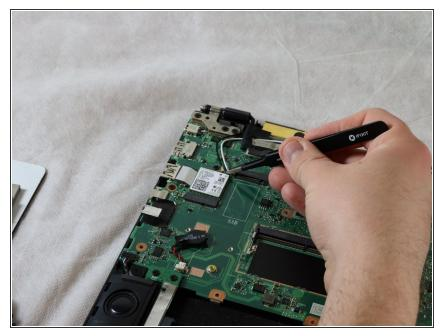
Use a pair of pointed tweezers to disconnect the small black and white coaxial connectors from the Wi-Fi card.
