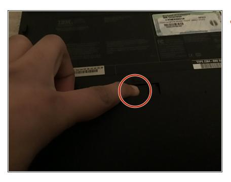
Turn over the laptop. Press the latch to remove the battery.
