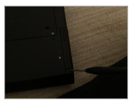
Remove the screw on the bottom next to the hard drive. It is under the palmrest on the side opposite the battery.
