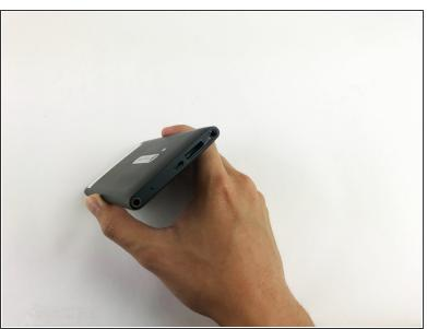
Insert the pointed end of the spudger into the sim card port indicated by the picture. Then proceed to remove the sim card port entirely.
