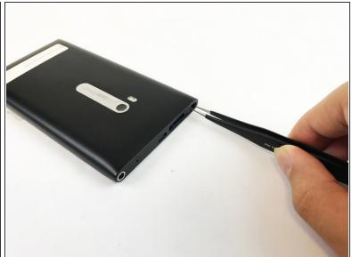
Use tweezers to remove the small rod in the port indicated in the picture.
