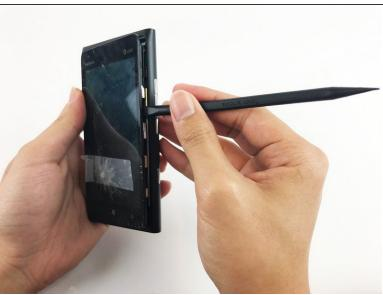
Separate the screen from the motherboard by prying it open with the spudger along with pulling upwards with the suction cup.
