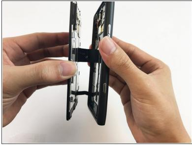
Gently pull apart the screen from the motherboard, with only the ribbons connected from the motherboard to the screen.
