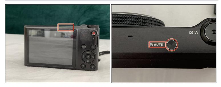
• Turn on the device by pressing the button thats labeled **POWER** on the top.
