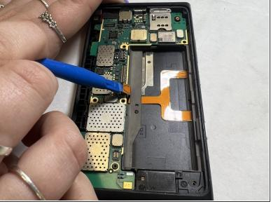
Use the plastic opening tool to lift the orange ribbon cable from the motherboard.
