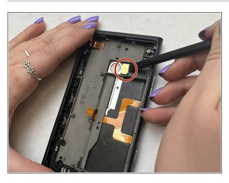
Use the flat end of a spudger to lift the LED out of the casing.
