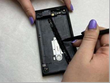
Wedge the pointed end of the spudger into the gaps in the antenna housing and pull the antenna housing away from the casing walls.
