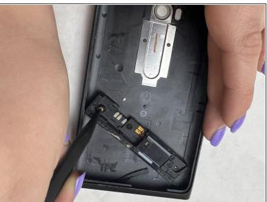
Insert the pointed end of the spudger into the hole and slide the speaker housing out from the casing.
