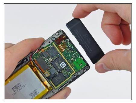
• Carefully slide the lower rear panel away from the Zune.
