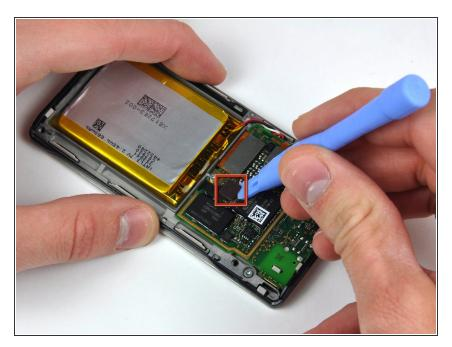
• Use a Zune opening tool to pry the digitizer ribbon cable connector up off the logic board.
