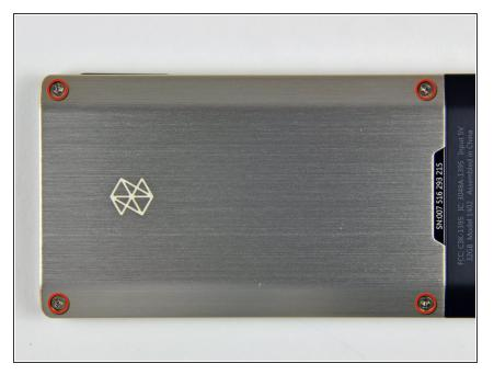
Remove the four Tri-Wing screws securing the upper rear panel to the inner chassis.
