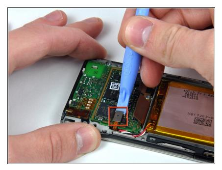
Use a Zune opening tool to pry the control ribbon cable up off the logic board.
