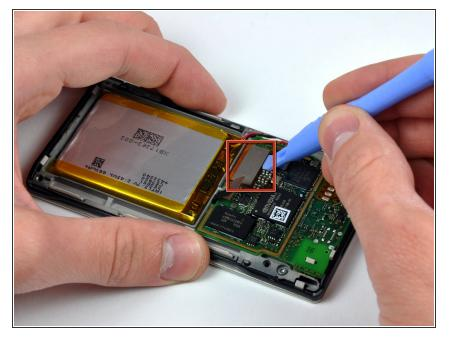
• Use a Zune opening tool to pry the OLED display ribbon cable connector up off the logic board.
