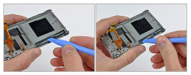
• Use a Zune opening tool to gently lift the media button lever off the post cast into the inner chassis.
