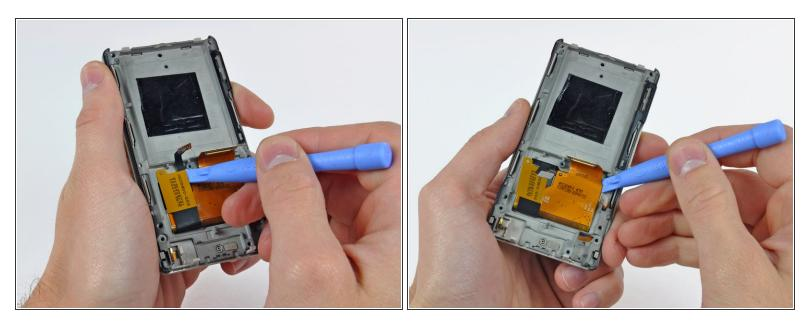
Use a Zune opening tool to peel the digitizer and display ribbon cables off the foam tape securing them to the inner chassis.
