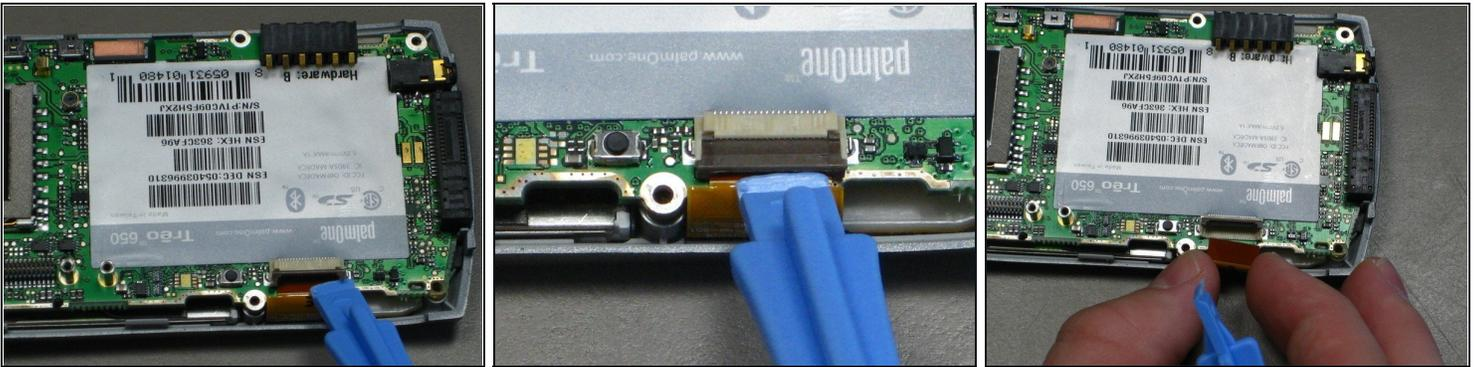
**⚠** Disconnect the ribbon cable before removing the motherboard.
