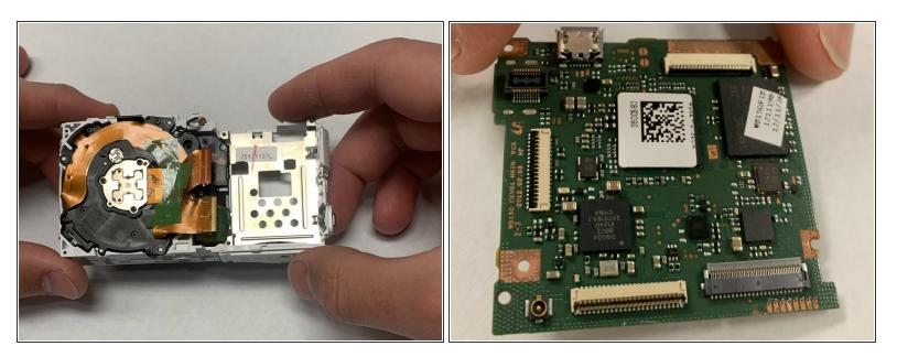
Remove the motherboard from the camera housing.
