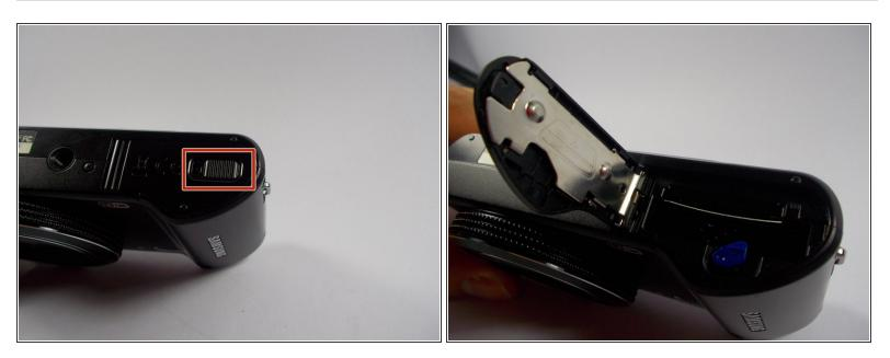
Have the lens of the camera face you. To open the battery compartment, slide the battery door lock towards the left. At the same time allow the battery door to swing open.
