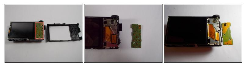
• On the screen side, remove the button circuit board (outlined in red) from the camera by using the plug located in the upper right corner of the screen side.
