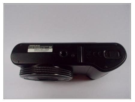
The location of the battery compartment can be found on the underside of the camera.
