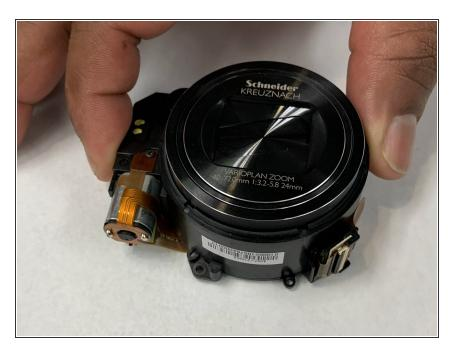
Lens assembly freely detaches from housing once both ribbons are detached from the motherboard.
