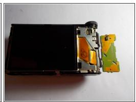
On the screen side, remove the button circuit board (outlined in red) from the camera by using the plug located in the upper right corner of the screen side.
