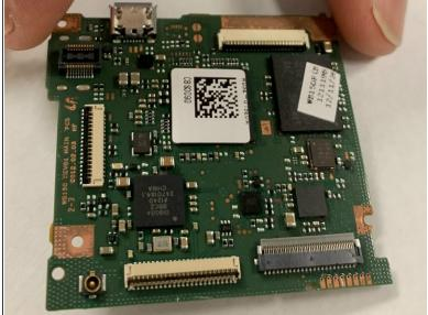
Remove the motherboard from the camera housing.
