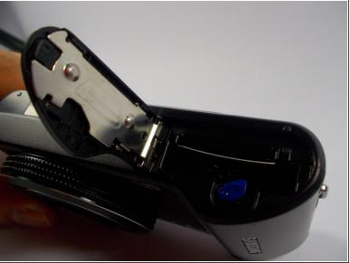
Have the lens of the camera face you. To open the battery compartment, slide the battery door lock towards the left. At the same time allow the battery door to swing open.
