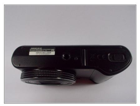
The location of the battery compartment can be found on the underside of the camera.
