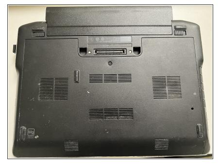
Flip the laptop over, so that the latches next to the battery are visible.
