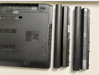
Carefully lift the back of the battery and take it out of the laptop.
