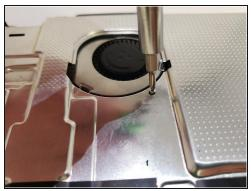
Locate the six Phillips head #00 screws from the metal plate inside of the device and remove them
