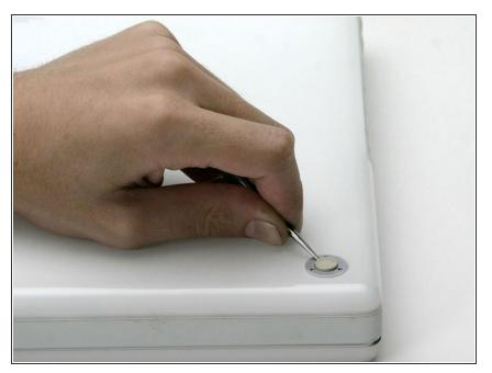
• Use a pin to remove the three rubber feet from the lower case.
