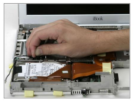
• Use the black plastic handle to disconnect the display data cable from the logic board.
