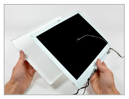
Lift the rear bezel off the display.
