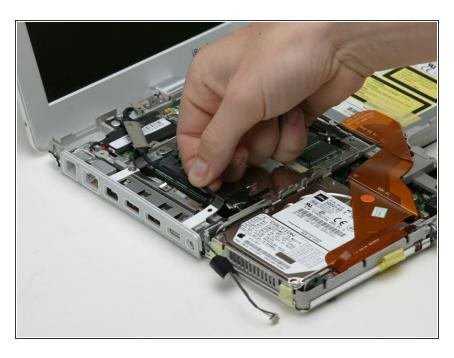
Deroute the display data and microphone cables.
