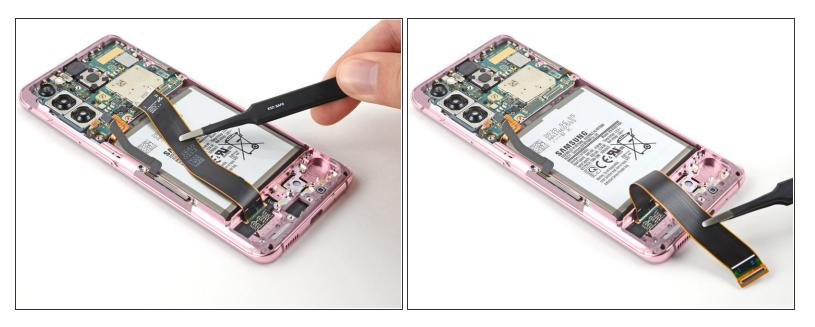
Gently peel up and bend the display flex cable out of the way of the motherboard and battery.
