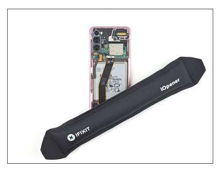
Apply a heated iOpener to the bottom-right corner of the device for 90 seconds.
