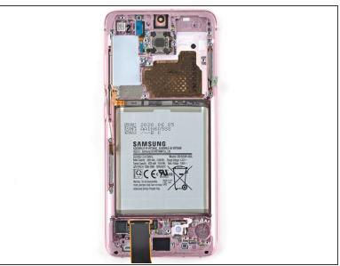
Use a Phillips screwdriver to remove the three 3.4 mm-long screws securing the 5G mmWave antennas.
