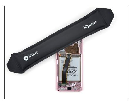
Heat an iOpener and apply it to the proximity sensor for two minutes.
