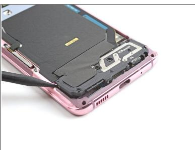
Insert the point of a spudger into the notch in the top left corner of the midframe and pry up to release the clips holding it in place.
