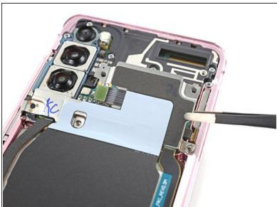
Use a pair of blunt-nose tweezers to gently pull up and unclip the motherboard bracket from the plastic midframe.
