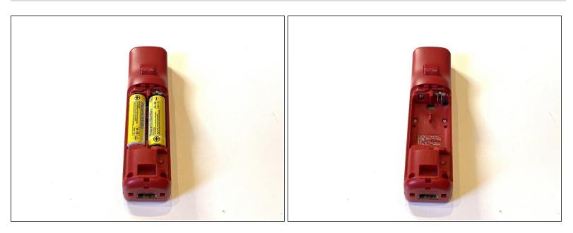
• Remove the battery using a fingernail.
