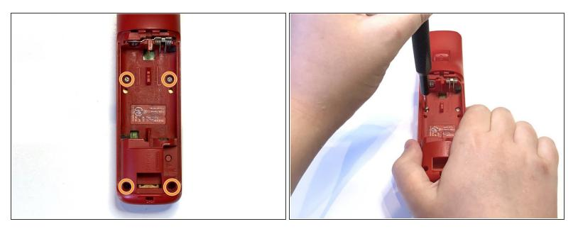
• This is where the disassembly begins, Grab your Y1 Screwdriver and unscrew the following screws
