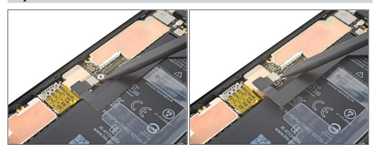
• Use a spudger to pry up and disconnect the 5G mmWave antenna's press connector.
