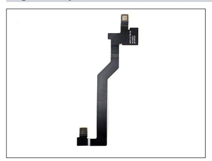
You're now left with the 5G mmWave antenna cable. Compare your new replacement part to the original part—you may need to transfer remaining components or remove adhesive backings from the new part before you install it.
