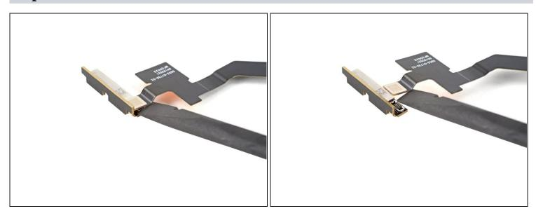
• Use a spudger to pry up and disconnect the 5G mmWave antenna cable's press connector.
