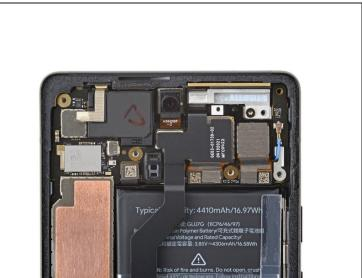
• Use a T3 Torx screwdriver to remove the 2.9 mm screw securing the 5G mmWave antenna bracket.
