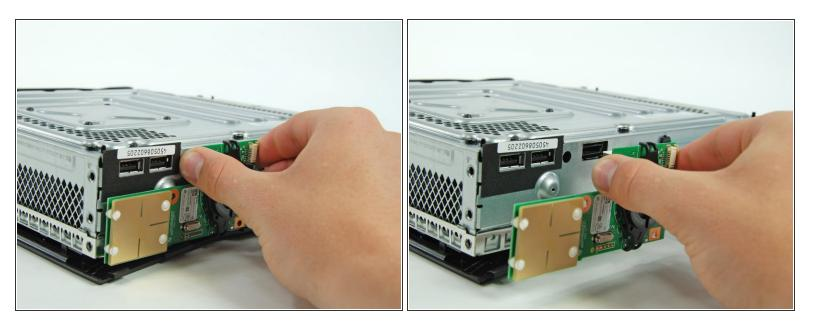
(i) The RF module is still connected to the Xbox by a large USB-type connector.
