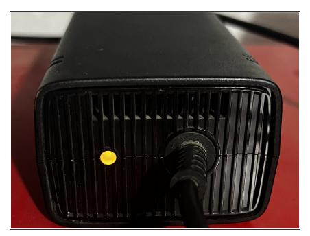
First things first, check the power supply. When plugged into the wall but not plugged into the unit, it should emit an orange light (showing that it is in standby mode). This light should stay orange when plugged into the unit. If it turns red, you likely have a PSU fault.
