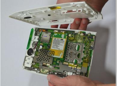
Start at one side of the device. Use a soft plastic prying tool to separate the casing of the device.
