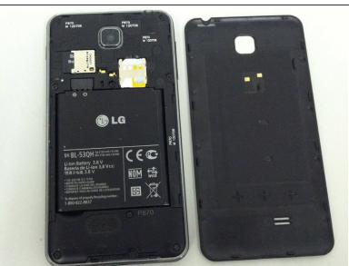
• Turn the device over and pull the back plastic cover off by inserting your fingernail into the opening at the bottom of the phone and gently pulling.
