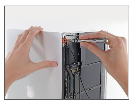
While holding the Air steady, remove the remaining 4.9 mm T8 Torx screw from the left display bracket.
