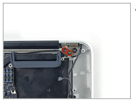
Remove the two 4.9 mm T8 Torx screws securing the antenna cable retainer on the left display hinge to the upper case.
