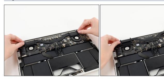
• Lift and remove the heat sink up off the logic board assembly.
