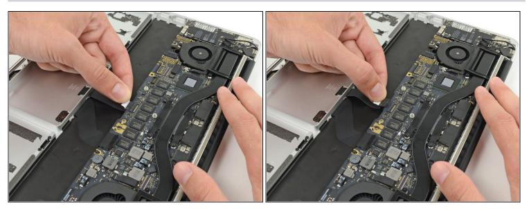
• Grasp the plastic pull tab and pull the trackpad ribbon cable out of its socket.
