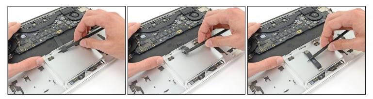
• Using the tip of the spudger carefully thread the trackpad ribbon cable out of the notch near the top of the SSD assembly cavity.
