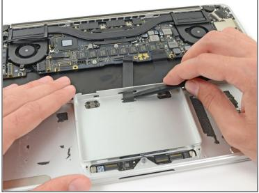
• Insert the tip of a spudger in between the trackpad ribbon cable and the upper case inside the SSD assembly cavity to remove the last of the adhesive.
