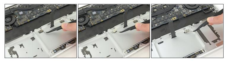
Use tweezers to remove the two trackpad mounting brackets from the upper case.
