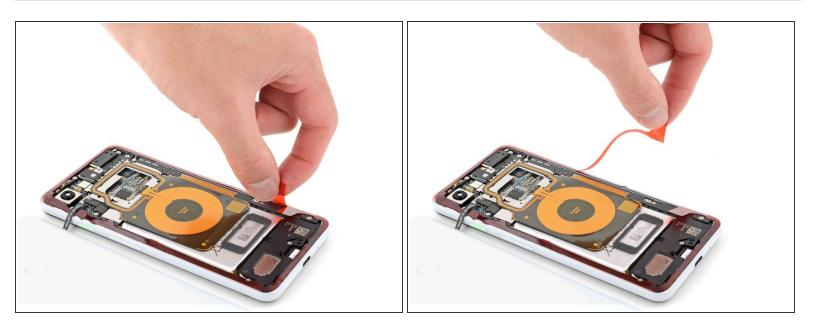
Peel away the red plastic lining to expose the back cover side of the adhesive.
