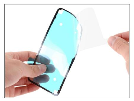
Peel away the clear plastic lining to expose the frame side of the replacement adhesive.
