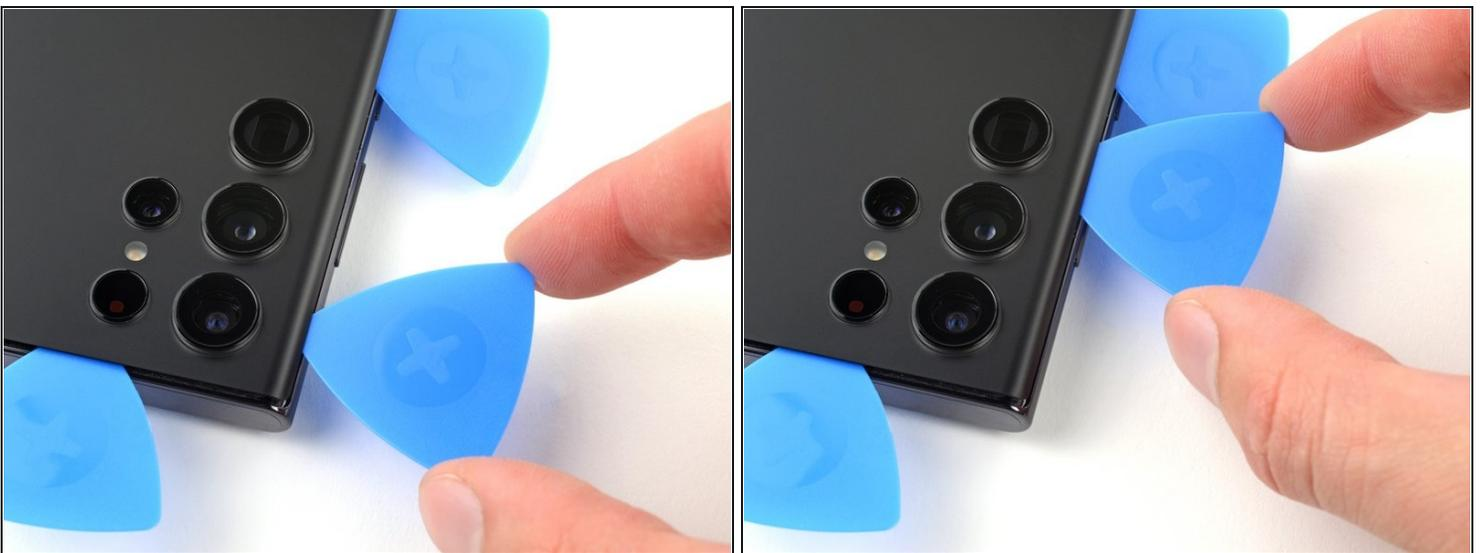
**⚠️ Only insert the pick up to 4 mm, as you may damage the cameras.**
