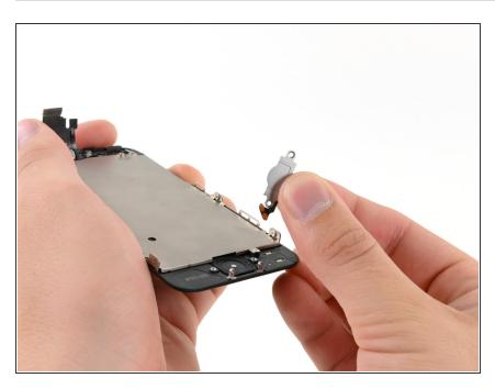
Remove the Home button shield and the cable.
