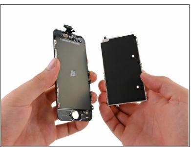
Remove the LCD screen shield.
