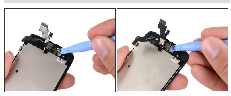
• In the position shown in the picture, there is a small cable connector, which can be gently removed with a plastic tool.
