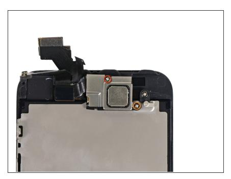
Remove the two screws as shown.
