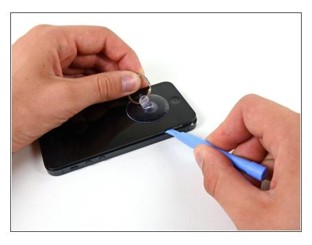
Slowly lift the buckle along the fuselage with a plastic ignition tool.
