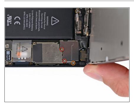
Unscrew the three screws as shown.
