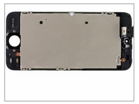
Unscrew the two screws as shown.
