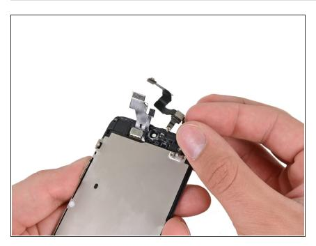
After you open the interface, you can remove the front camera.
