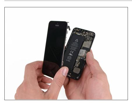
After disconnecting these three interfaces, now you can remove the screen.
