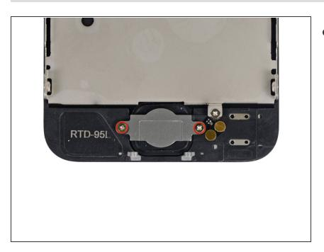
Unscrew the two screws as shown.
