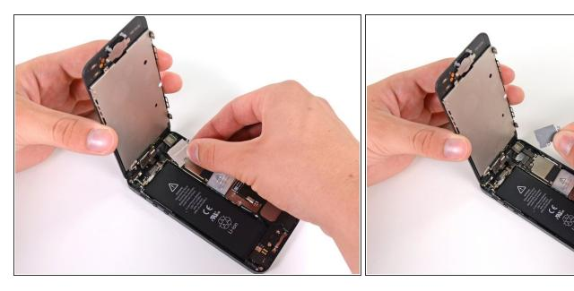
Remove the small baffle.
