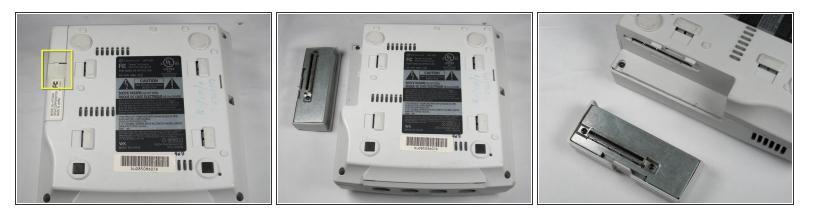
• **Remove the expansion bay** by applying pressure to the small clip on the expansion bay while prying it away from the console.
