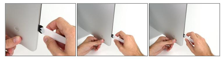
• Starting on the left of the display, near the power button, insert the iMac Opening Tool into the gap between the glass panel and the rear case.
