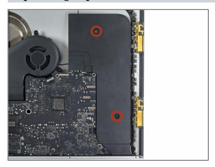
Remove two 10.0 mm T10 screws.
