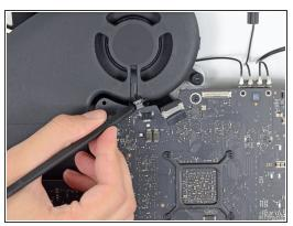
• Use the tip of a spudger to disconnect the fan cable's connector from its socket on the logic board.
