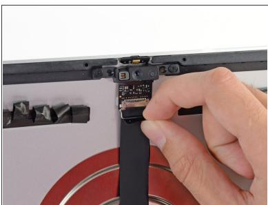
Flip down the metal retaining bracket on the iSight camera cable.
