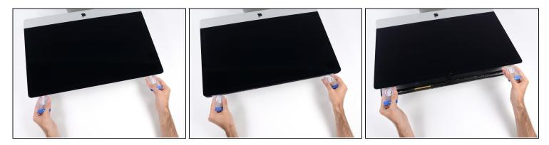
⚠ Only lift the display a few inches—it is still attached to the iMac by data and power cables.
