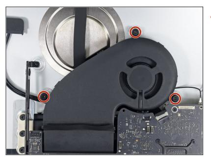
• Remove three 12.4 mm T10 screws securing the fan to the rear case.
