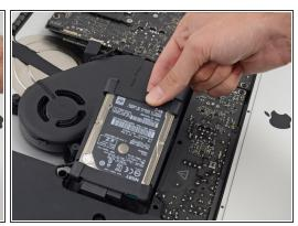
Lift the hard drive from the edge nearest the fan and pull it slightly out of its recess.
