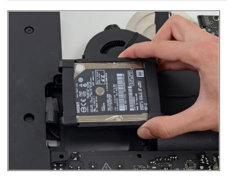
Lift and remove the hard drive from the iMac.
